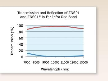
Transmission values are on a multispectral Zinc Sulphide substrate which has been coated on both surfaces with ZNS-01
